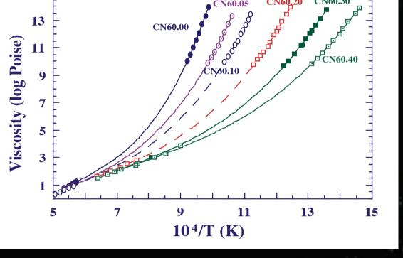
Figure 1 : Viscosity data of the soda-lime silicate glasses and melts as a function of reciprocal temperature
