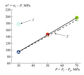
**Fig. 2.** Uniaxial compressive strength of specimens  $\sigma^*$  as function of effective pressure of uniform compression *P* (difference of uniform compression pressure and pore pressure) in experiments BS02 (circles) and BS03 (triangles). Colors correspond to curves 5 in Fig. 1. *I*, intact specimen at preparatory stage; *2*, specimen with formed macrofracture at working stage. For stage *2*, regression lines are shown: solid line for BS02 and dashed line for BS03.
