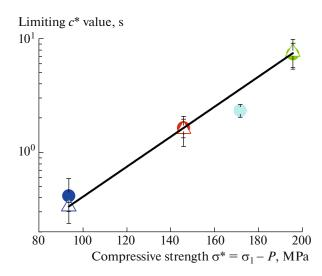
Fig. 5. Dependence of limiting values of Omori parameter  $c^*$  on compressive strength. Colors of points correspond to curves 5 in Fig. 1, experiments BS02 (circles) and BS03 (triangles). Straight line shows exponential approximation (9).
