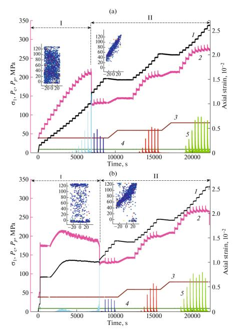
Fig. 1. Loading history in experiments (a) BS02 and (b) BS03: 1, axial strains; 2, axial stresses  $\sigma_1$ ; 3, uniform compression pressure  $P_c$ ; 4, pore pressure  $P_p$ ; 5, acoustic activity (different colors show activity at different values of uniform compression pressure). Insets show examples of distributions of acoustic emission sources within specimens at preparatory (I) and working stages (II).
