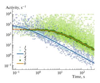
**Fig. 3.** Examples of decay of acoustic activity for different levels of axial stresses  $\sigma_1$  and uniform compression pressure *P* (experiment BS02): *1–3*,  $\sigma_1$ = 134 MPa, *P*=40 MPa; *2–4*,  $\sigma_1$  = 275 MPa, *P* = 80 MPa; *1*, *4*, disaggregated values; *2*, *5*, values aggregated over 100 events within moving window shifted by 20 events; *3*, *6*, approximation according to Modified Omori law (1).
