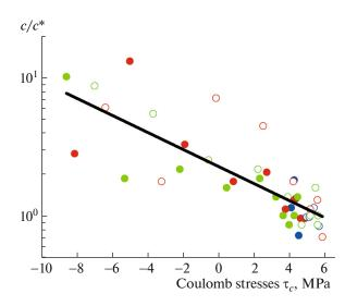
**Fig. 6.** Omori parameter *c* normalized to  $c^*$  corresponding to ultimate strength. Colors of points correspond to curves 5 in Fig. 1, experiments BS02 (circles) and BS03 (triangles). Regression line according to (10) is shown.
