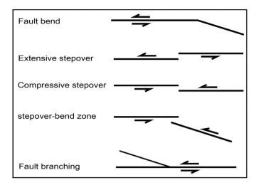
Fig. 19. Typical geometric complexities along a left-lateral strike-slip fault: fault bend (fault azimuth change), jog or relay zone or stepover that can be extensive or compressive, stepover-bend zone (a combination of the two previous cases), and fault branching.
