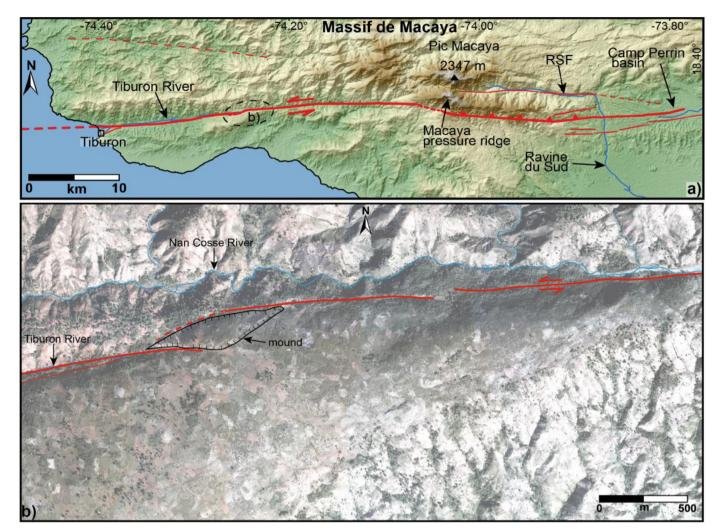
**Fig. 12.** a) Topographic map of the areas of Macaya and Tiburon River. The Pic Macaya (2347 m) is out the area of bordering faults. The Macaya pressure ridge is to the south of the peak (see text for discussion). RSF: Ravine du Sud Fault. The black dotted ellipse is the location of (b). b) Aerial photograph (pixel: 30 cm) of Nan Cosse River. Almost the whole southern wall of that river is encroached by the EPGF. The mound is discussed in Section 5.
