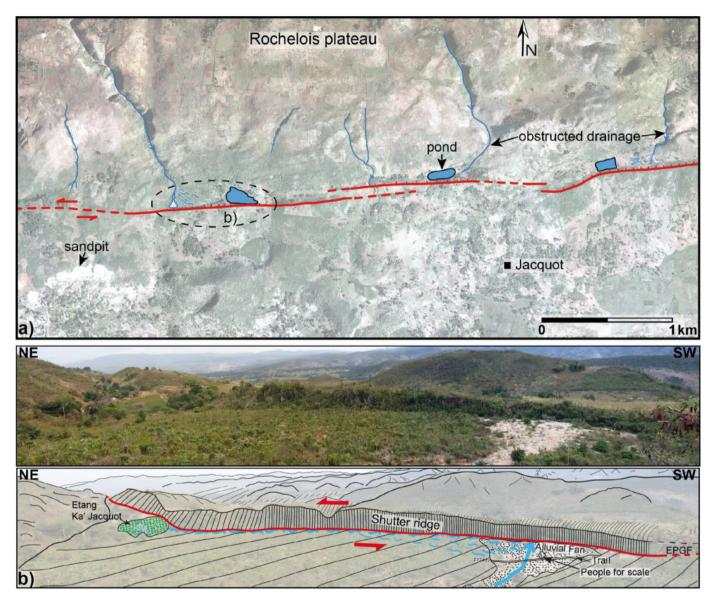
**Fig. 9.** a) Aerial photograph (pixel: 30 cm) of Jacquot area. The south-flowing drainages are deflected or obstructed by the fault. The streams pond in front of the fault scarp as shown by the basins. The dotted ellipse locates (b). b) Field photo mosaic and interpretation of Etang Ka' Jacquot (Ka' Jacquot pond) area. The drainage abuts against a  $\sim$ 10-m fault scarp that acts as a shutter ridge.
