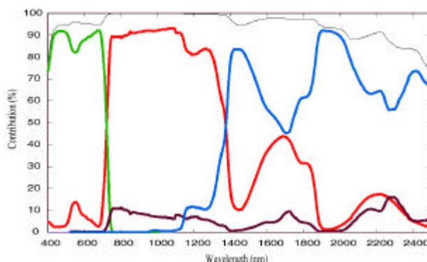
Figure 4. Contribution of chlorophyll concentration  $C_{ab}$  (green), equivalent water thickness  $C_w$  (blue), dry matter content  $C_m$  (brown) and structure parameter  $N$  (red) to the leaf transmittance as simulated by PROSPECT. The black curve is the sum of the contributions (Pavan, unpublished).
