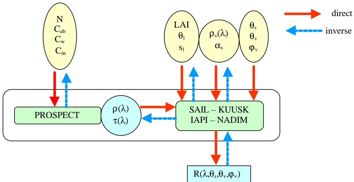
Figure 6. Schematic representation of the PROSPECT + SAIL (or any other canopy reflectance model) model, in direct and inverse modes.
