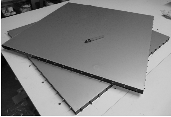
Fig. 4. View of two 16 \times 16 matrices. The optical plugs are visible on two sides of each matrix and are to be connected to the clear fibers guiding the light onto the channels of the photomultiplier. The thickness of the matrices is 27 mm and their individual total weight is 20 kg.
