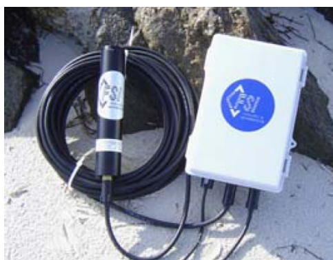
Figure 5. Capteur FALMOUTH SCIENTIFIC EOPM « High accuracy self-contained tide recorder » (photo http://www.falmouth.com )
